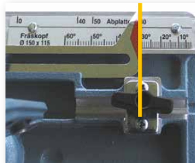
Just position the machine on the skew notch edge of reference.
