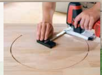
Compass saw functionality (50 mm - 210 mm radius)
