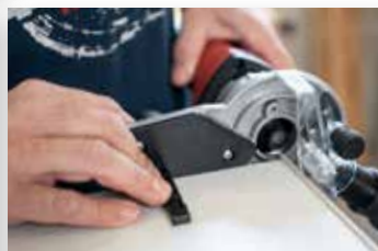
Plug-in fence serves as reliable guide when machining corners.
