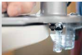
With sensitive materials, a friction ring brake prevents ugly machining marks.
