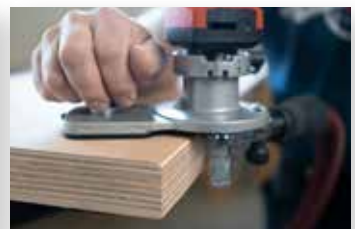
Even solid wood edges can be machined with commercially available cutters.
